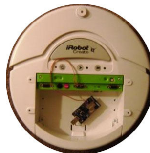
Figure 2. The configuration between iRobot and Tmote Sky sensor.
